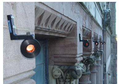
Above: L-shaped prism on a building
