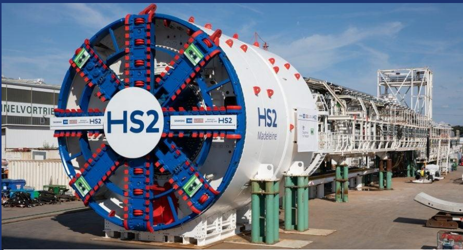
TBM Madeleine at the Herrenknecht factory in Germany
