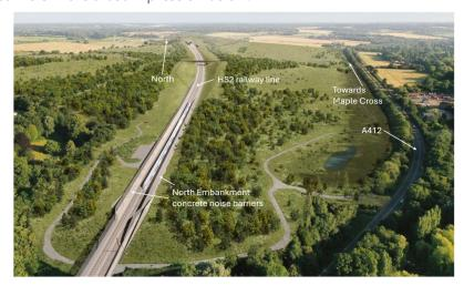
In March this year we will also begin the final stages of the landscaping, which will include vegetation clearance, removal of the North Embankment compound, constructing the North Embankment access road for railway maintenance vehicles; topsoiling and planting; the restoring of the Old Shire Lane footpath and new access from the A412, as well as new bridleways and a viewing area.
