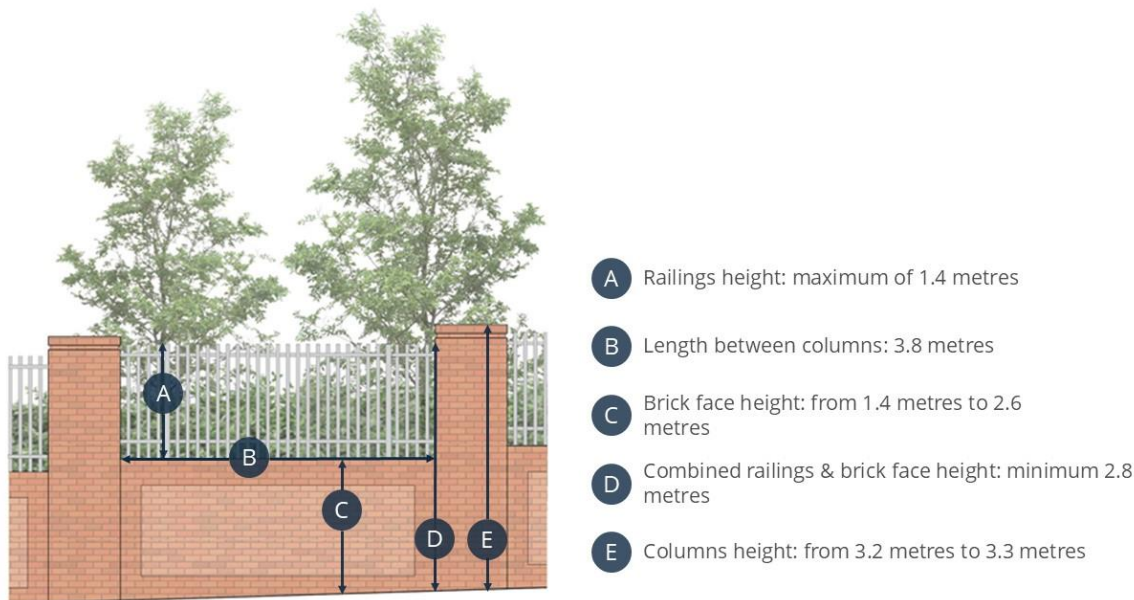
Figure 2: Permanent compound wall design with dimensions
