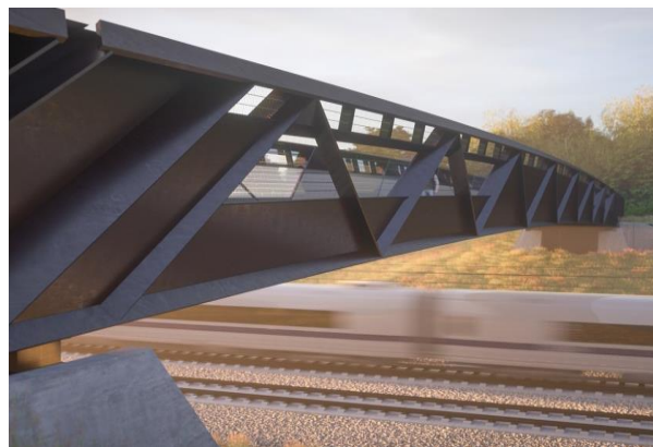
Figure 7: The CGI above show, the HS2 rural footbridge design from the side with passing train below.
