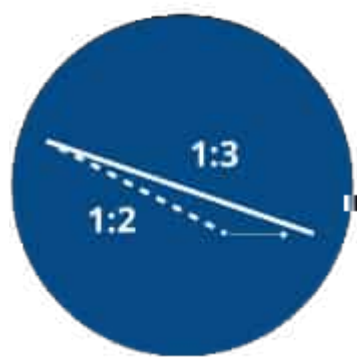
Step 3 Earthwork gradient
