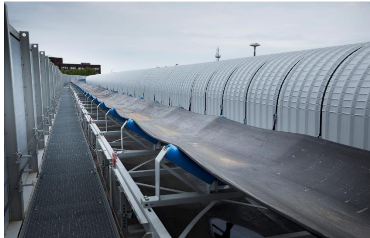
Installation of conveyor belt and dust covers in Flat Iron site in September 2022
