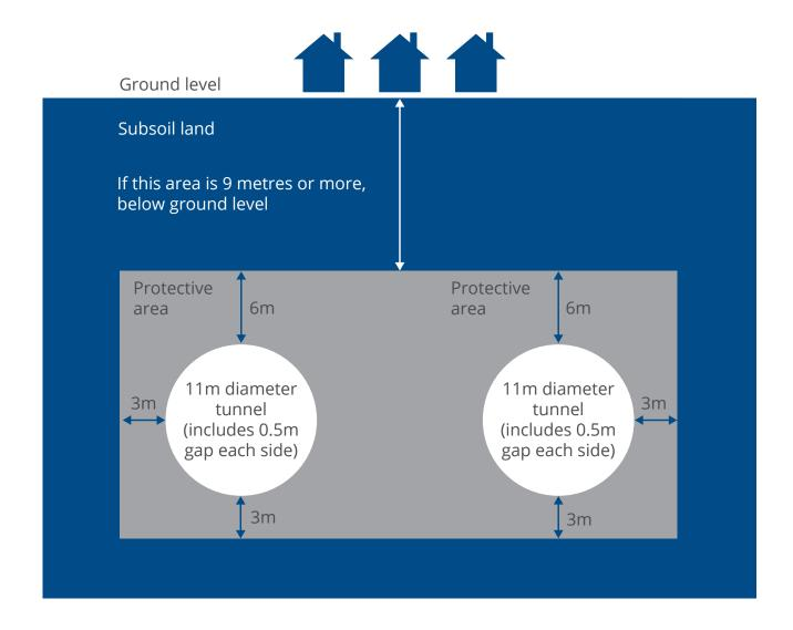
We will use an area of subsoil outside the tunnel limits as a protective area to maintain the long-term safety of the railway. The size of the protective area may alter for each tunnel to avoid conflicting with existing structures.
