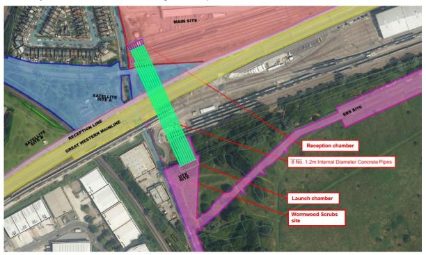
The above image shows the site working area with the eight green lines showing the micro-tunnels running from Wormwood Scrubs to the main site
