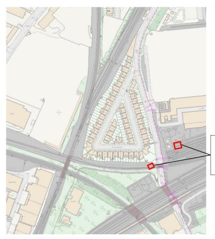
A crawler crane and piling rig will be operational in these locations to install piles ahead of the conveyor installation
