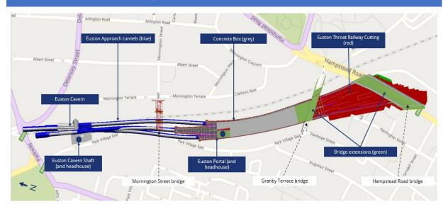
To build the supporting structures for the tunnels and the future HS2 railway in Euston Approaches, we will also carry out other major excavations. This involves digging out large volumes of earth several metres below the current ground level and removing the spoil by lorries. Removal by rail is not possible in this location without causing unacceptable disruption to existing rail services.
