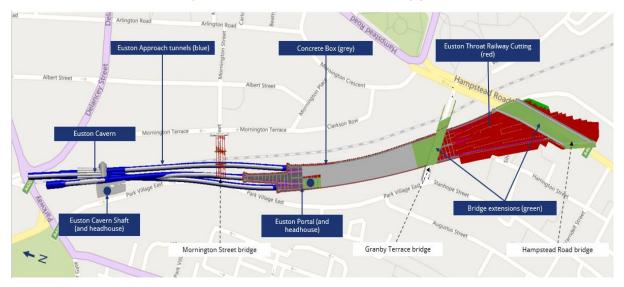
To build the supporting structures for the tunnels and the future HS2 railway in Euston Approaches, we will also carry out other major excavations. This involves digging out large volumes of earth several metres below the current ground level and removing the spoil by lorries. Removal by rail is not possible in this location without causing unacceptable disruption to existing rail services.
