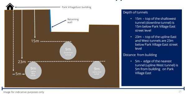
We will excavate the three tunnels and spray them with a concrete lining. This is a tried and tested method on major tunnelling projects known as sprayed concrete lining (SCL) tunnelling. This involves excavating a very small section of tunnel with diggers and then immediately lining it with concrete before moving forward and repeating the process.
