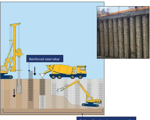
Guide wall and continuous secant piles
