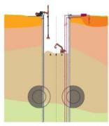
The ground around the tunnel entry points is prepared for the arrival of the Tunnel Boring Machines (TBMs). Earth is removed from within the walls with excavators. Groundwater in the shaft is pumped out to local recharge wells.
