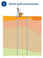
The outer walls of the vent shaft are created using Diaphragm Walls (or 'D'-Walls). These are constructed from the ground level (top-down). This protects the excavation work from lateral earth pressure and water pressure. These walls will form the external structure of the finished vent shaft.
