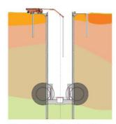
The outer walls of the headhouse are constructed using a technique called secant piling. When the earth from within the shaft walls has been excavated, concrete is poured into the shaft to create the base slab. A structure called a collar is constructed to support the shaft when the TBMs arrive and pass through.
